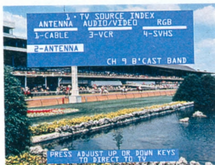
Switch between different signal inputs with the TV source index
